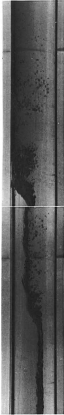
(a) Typical back of a gas cavity in the slug flow ( U_{SG} = 1.45 m/s; U_{SL} = 0.95 m/s; Fr = 2.53 ).
